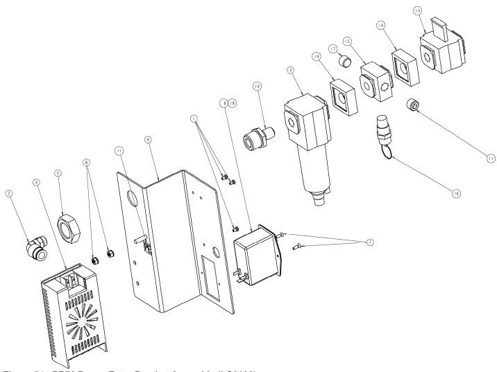
Figure 54: PR70 Power Entry Bracket Assembly (LC0106)
